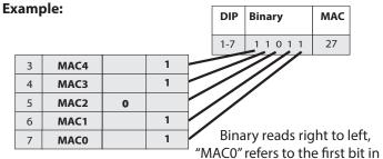
the binary string, from there the dip switches are set following the description ordering using the binary string for the desired setting. In this example the full binary string for 27 is 0011011, switch "MAC5" and "MAC6" would be turned off.
