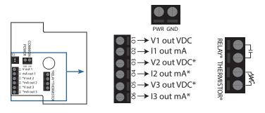
Outputs 1(V1,I1), 2(V2,I2) and 3(V3,I3), will be auto populated in order of the AQ2W ordering matrix: CO2, RH, Temp, VOC, PM, Slider, CO, O3
